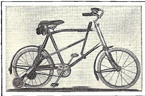
Two safety wheels attached to the rear axle of this new bicycle make it safe for the youngster learning to ride. The lever, mounted forward of the seat, may be shifted, raising wheels from the ground to form an ordinary bike.
