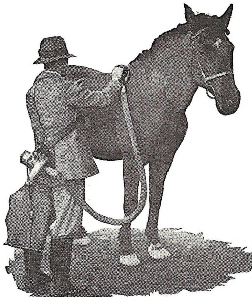
Photo shows horse being "vacuum cleaned" with new electrical curry comb. Dirt is drawn through hose into bag.
