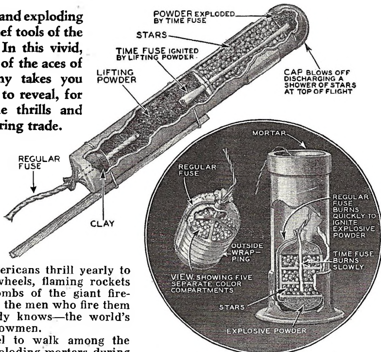
Top drawing shows cross section of giant rocket that discharges star showers. Below is mortar and bomb which is divided into sections holding the different colored stars.
